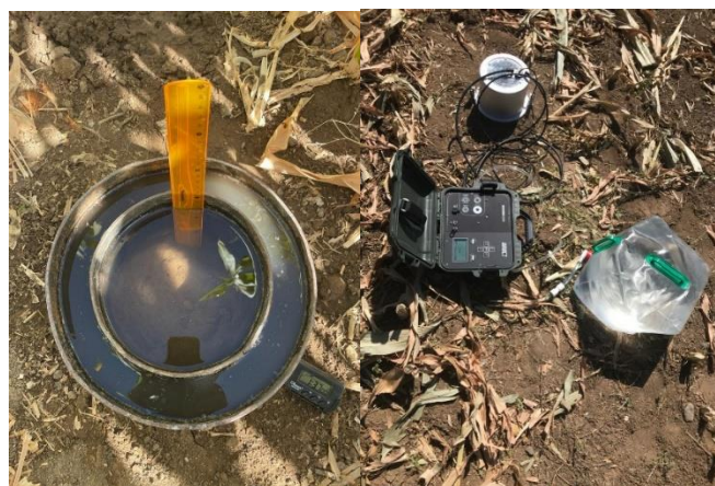
Figure 1. Infiltration measurements with automatic infiltrometer and double ring infiltrometer
