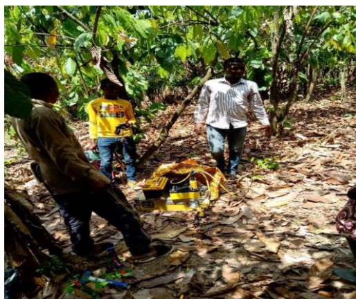
Figure 2a: Geophysical Crew Deploying ERT meter
